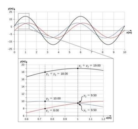
When two linear waves in the same medium interfere, the height of resulting wave is the sum of the heights of the individual waves, taken point by point. This plot shows two waves (red and blue) added together, along with the resulting wave (black). These graphs represent the height of the wave at each point. The waves may be any linear wave, including ripples on a pond, disturbances on a string, sound, or electromagnetic waves.
