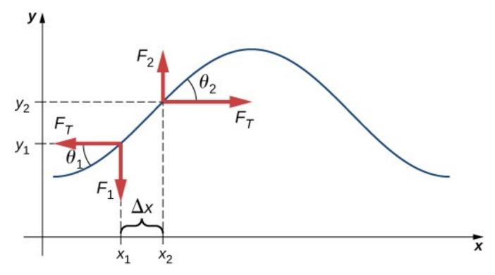
A string under tension is plucked, causing a pulse to move along the string in the positive *x*-direction.
