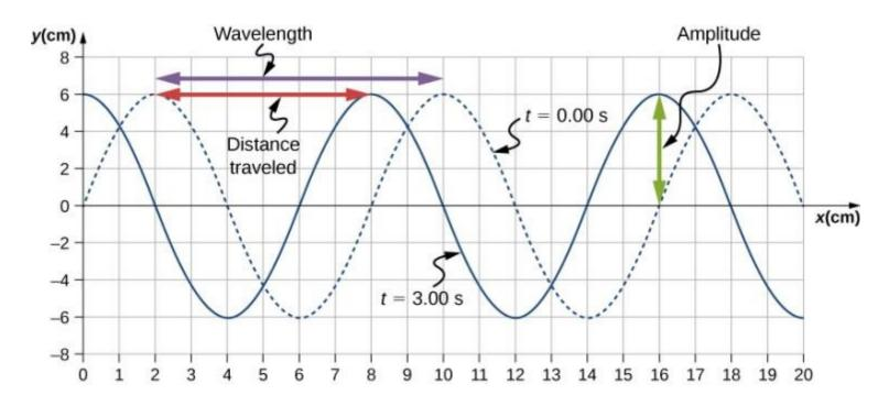
Characteristics of the wave marked on a graph of its displacement.
