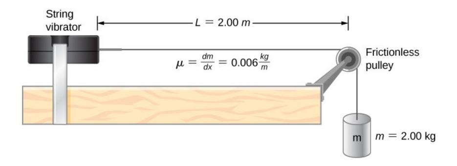
A string attached to an adjustable-frequency string vibrator.
