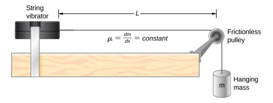
A lab setup for creating standing waves on a string. The string has a node on each end and a constant linear density. The length between the fixed boundary conditions is L. The hanging mass provides the tension in the string, and the speed of the waves on the string is proportional to the square root of the tension divided by the linear mass density.
