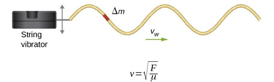
A string vibrator is a device that vibrates a rod. A string is attached to the rod, and the rod does work on the string, driving the string up and down. This produces a sinusoidal wave in the string, which moves with a wave velocity v. The wave speed depends on the tension in the string and the linear mass density of the string. A section of the string with mass m oscillates at the same frequency as the wave.
