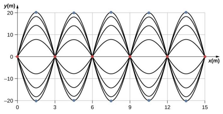
When two identical waves are moving in opposite directions, the resultant wave is a standing wave. Nodes appear at integer multiples of half wavelengths. Antinodes appear at odd multiples of quarter wavelengths, where they oscillate between  $y = \pm A$ . The nodes are marked with red dots and the antinodes are marked with blue dots.
