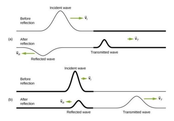
Waves traveling along two types of strings: a thick string with a high linear density and a thin string with a low linear density. Both strings are under the same tension, so a wave moves faster on the low-density string than on the high-density string.
