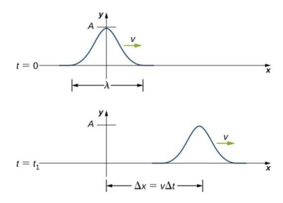
The pulse at time t = 0 is centered on x = 0 with amplitude A. The pulse moves as a pattern with a constant shape, with a constant maximum value A. The velocity is constant and the pulse moves a distance x = vt in a time t. The distance traveled is measured with any convenient point on the pulse. In this figure, the crest is used.
