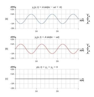
Destructive interference of two identical waves, one with a phase shift of 180°( rad), produces zero amplitude, or complete cancellation.
