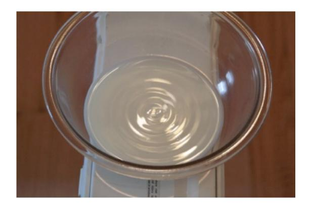
Standing waves are formed on the surface of a bowl of milk sitting on a box fan. The vibrations from the fan causes the surface of the milk to oscillate. The waves are visible due to the reflection of light from a lamp.
