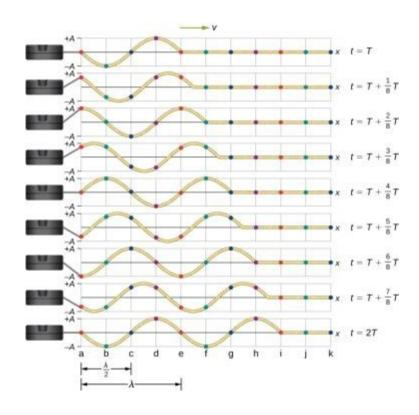
Snapshots of a transverse wave moving through a string under tension, beginning at time t = T and taken at intervals of . Colored dots are used to highlight points on the string. Points that are a wavelength apart in the x-direction are highlighted with the same color dots.
