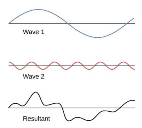
Superposition of nonidentical waves exhibits both constructive and destructive interference.
