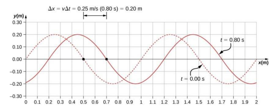
A graph of height of the wave y as a function of position x for snapshots of the wave at two times. The dotted line represents the wave at time t = 0.00 s and the solid line represents the wave at t = 0.80 s. Since the wave velocity is constant, the distance the wave travels is the wave velocity times the time interval. The black dots indicate the points used to measure the displacement of the wave. The medium moves up and down, whereas the wave moves to the right.
