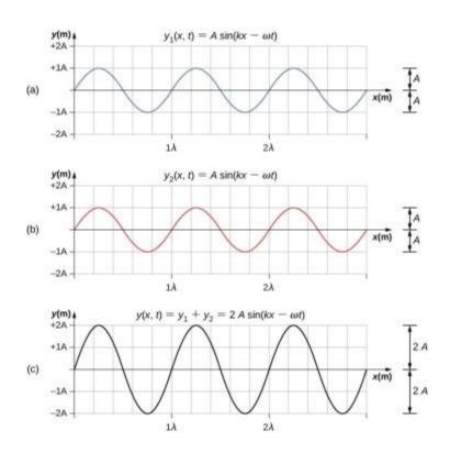
Constructive interference of two identical waves produces a wave with twice the amplitude, but the same wavelength.
