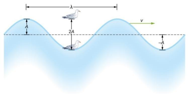
An idealized surface water wave passes under a seagull that bobs up and down in simple harmonic motion. The wave has a wavelength  $\lambda$ , which is the distance between adjacent identical parts of the wave. The amplitude A of the wave is the maximum displacement of the wave from the equilibrium position, which is indicated by the dotted line. In this example, the medium moves up and down, whereas the disturbance of the surface propagates parallel to the surface at a speed  $\nu$ .
