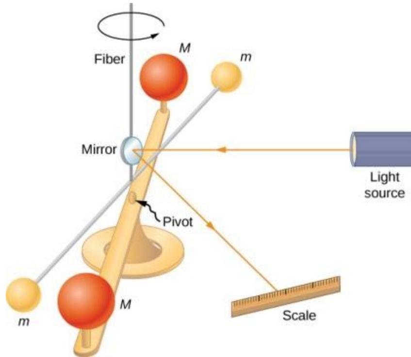
Cavendish used an apparatus similar to this to measure the gravitational attraction between two spheres ( $m$ ) suspended from a wire and two stationary spheres ( $M$ ). This is a common experiment performed in undergraduate laboratories, but it is quite challenging. Passing trucks outside the laboratory can create vibrations that overwhelm the gravitational forces.
