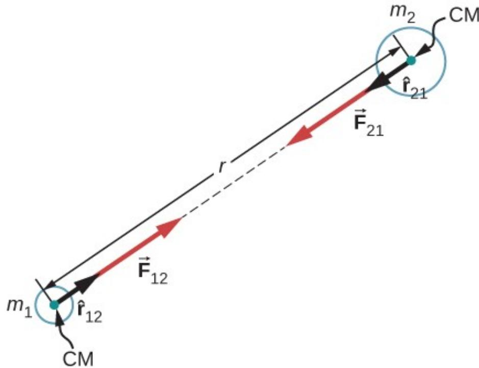
Gravitational force acts along a line joining the centers of mass of two objects.
