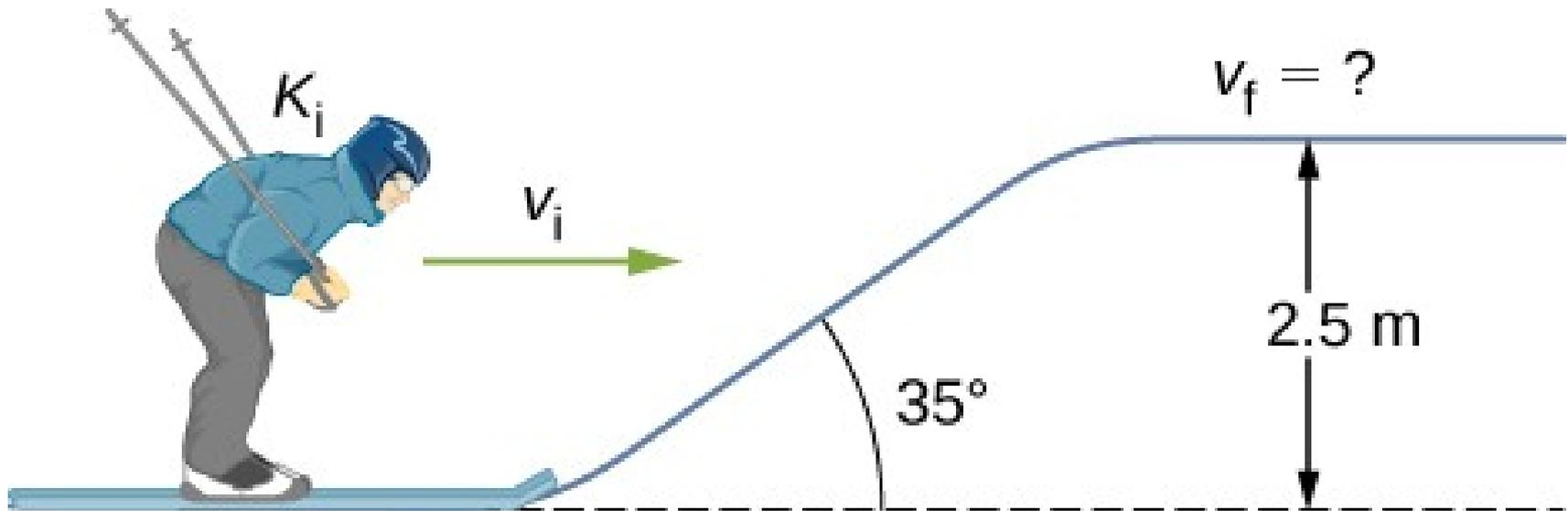
A skier with an initial speed of  $v_0$  coasts up a  $h$  high rise as shown. Find her final speed at the top, given that the coefficient of friction between her skis and the snow is  $\mu_k$ .
