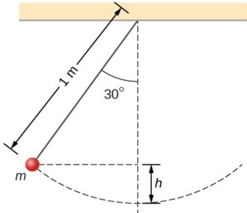
A particle hung from a string constitutes a simple pendulum. It is shown when released from rest, along with some distances used in analyzing the motion.
