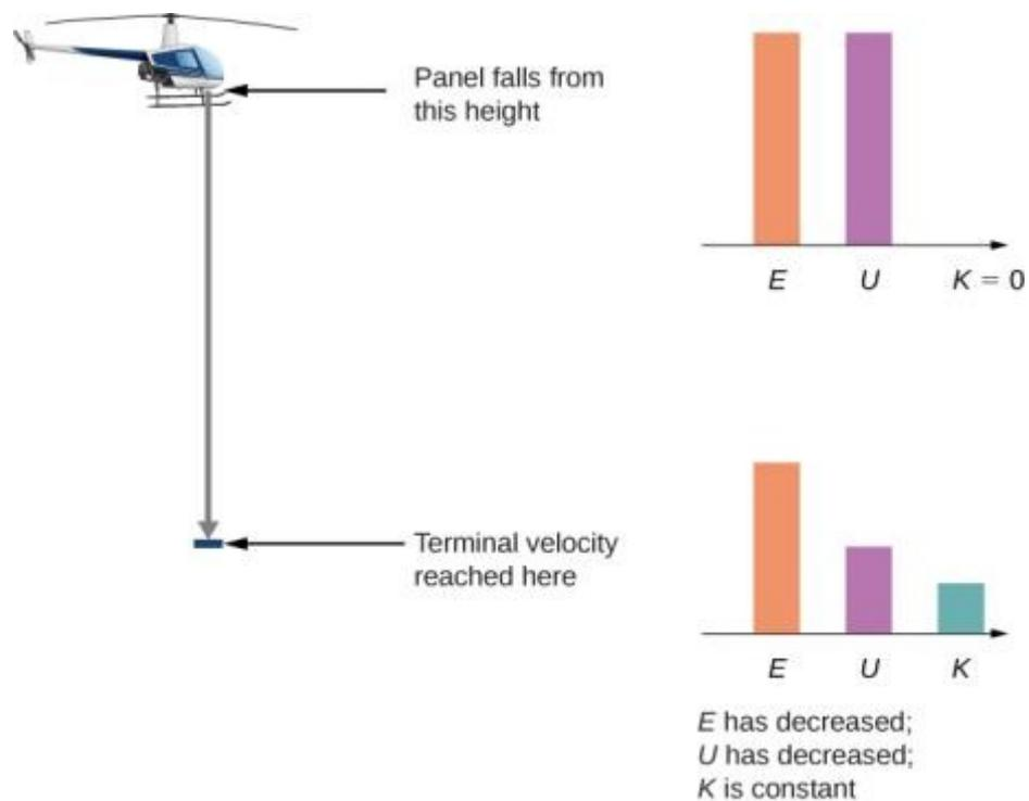
A helicopter loses a panel that falls until it reaches terminal velocity of 45 m/s. How much did air resistance contribute to the dissipation of energy in this problem?
