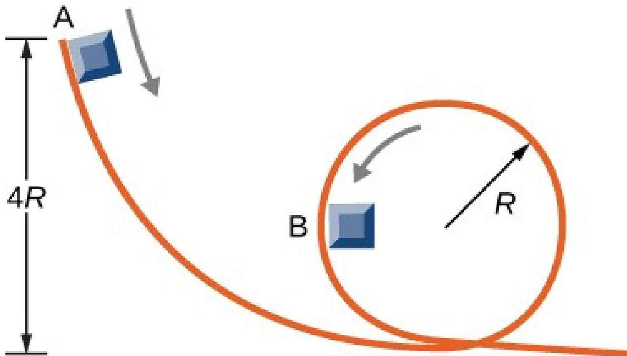
A small block of mass  $m$  slides without friction around the loop-the-loop apparatus shown below. (a) If the block starts from rest at  $A$ , what is its speed at  $B$ ? (b) What is the force of the track on the block at  $B$ ?
