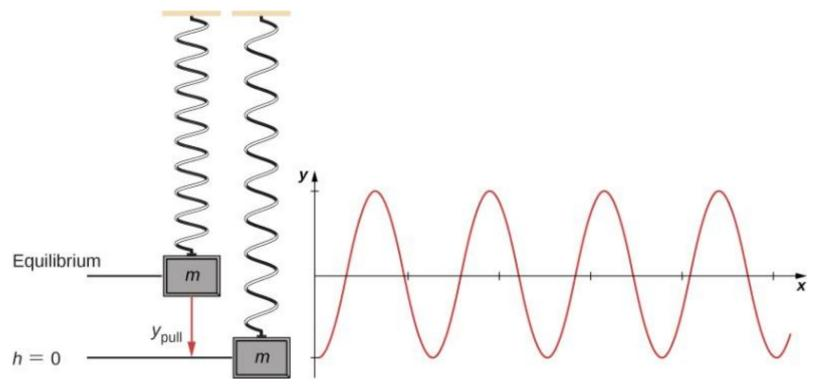
A vertical mass-spring system, with the y-axis pointing upward. The mass is initially at an equilibrium position and pulled downward to  $y_{\text{pull}}$ . An oscillation begins, centered at the equilibrium position.
