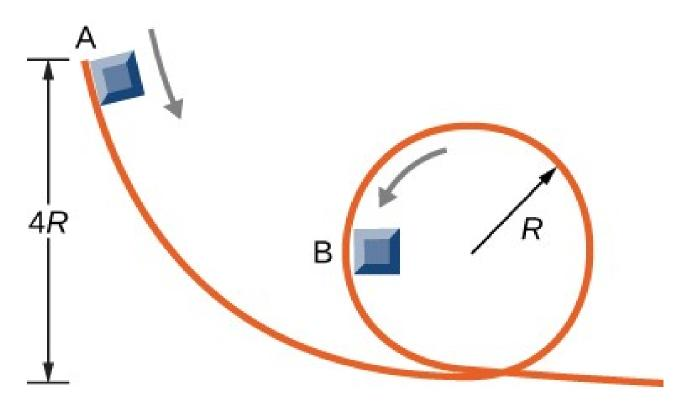
A small block of mass *m* slides without friction around the loop-the-loop apparatus shown below. (a) If the block starts from rest at *A*, what is its speed at *B*? (b) What is the force of the track on the block at *B*?
