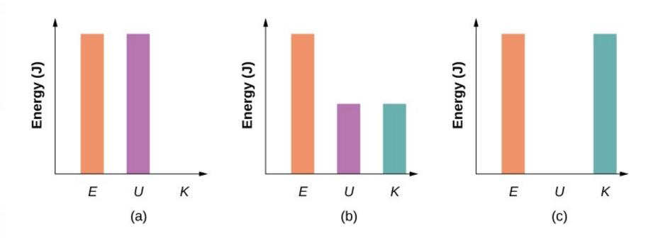
Bar graphs representing the total energy (E), potential energy (U), and kinetic energy (K) of the particle in different positions.
